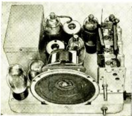
Above, chassis view of the new radio set. Right, schematic circuit of the receiver. Late tube types, including an 84, are used in an efficient circuit.
