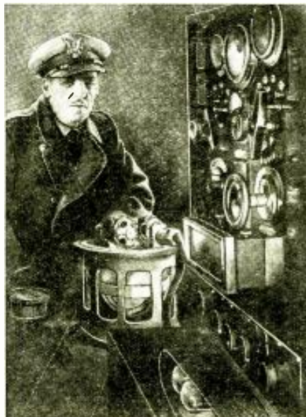
Fig. 4 Receiving apparatus shown on right, steering gyroscope in center.
