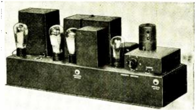
A typical small-theater amplifier, incorporating volume control, fader switch, and monitor jack.
